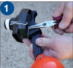
1 Remove small R-Pin that holds the pivot pin in place
