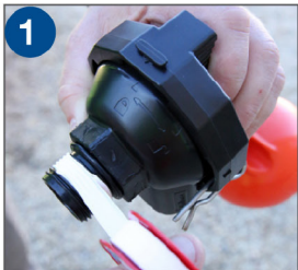
1 Apply PTFE tape in a clockwise direction
