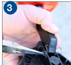
3 Unclip damper spring from cap
