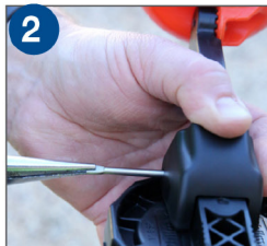
2 Remove pivot pin, dispose of spring cover
