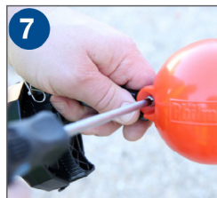
7 Using a Phillips head screwdriver unscrew Float
