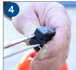
4 Remove spring retainer from float arm and remove damper spring
